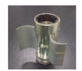
81 mm and 50 mm rocket engine pipes and vanes
